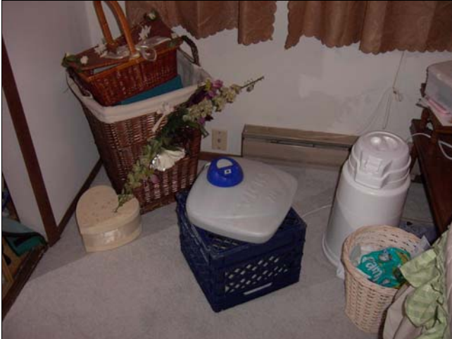
The second floor north bedroom had a humidifier. This apparatus could have easily contributed to augmented humidity levels in the attic.
