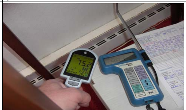
Diagnostics equipment showed the humidity showed that the register was not warm and the home heating system was not properly balanced.
