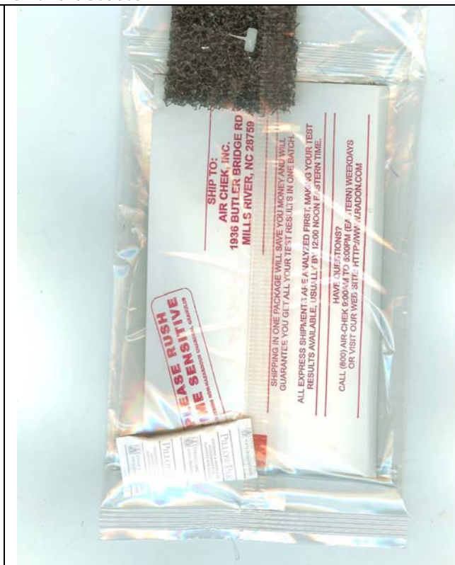
Back of detectors (Actual size is much bigger) All detectors come sealed in two plastic containers. Plastic is only removed when test is being deployed.
